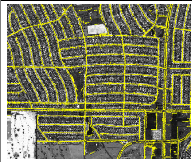
Figure 3. Streets centerlines automatically created from the polygons. During the convert-to-line process, small dangles are removed, gaps are jumped, intersections are cleaned, and the lines are smoothed using a line snake algorithm.
